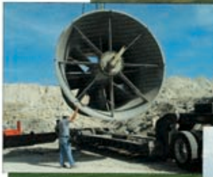
470 cfs pump for pump station
